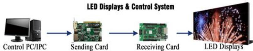
**LED Displays System Diagram**
